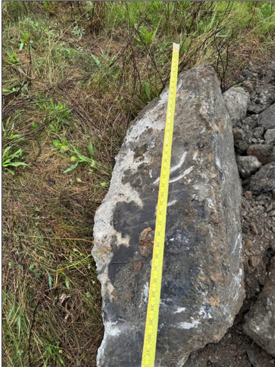
PHOTO NO. 4: Test Pit TP-6 with large concrete debris.
