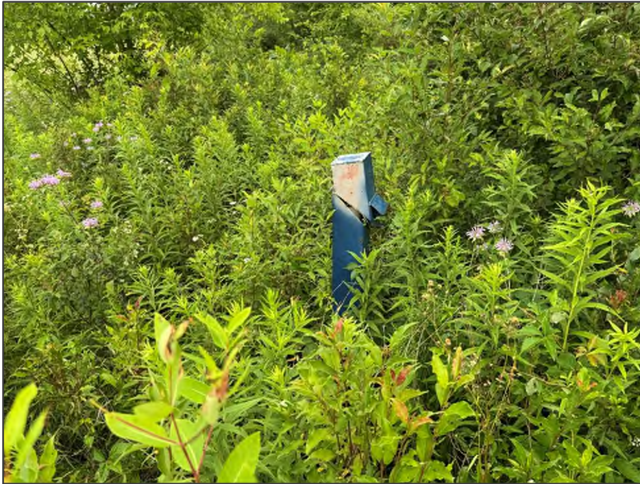
PHOTO NO. 9: View of a typical monitoring well on the Subject Property.
